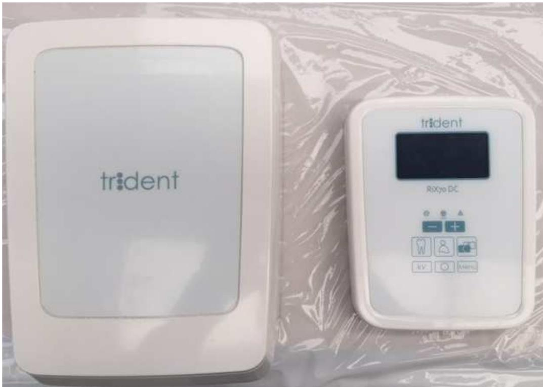
The remote timer is connected directly to the driver board through a coaxial Ethernet cable(not included in the package, you must buy the cable according to your needs). During the installation, the cable needs to be already connected.
