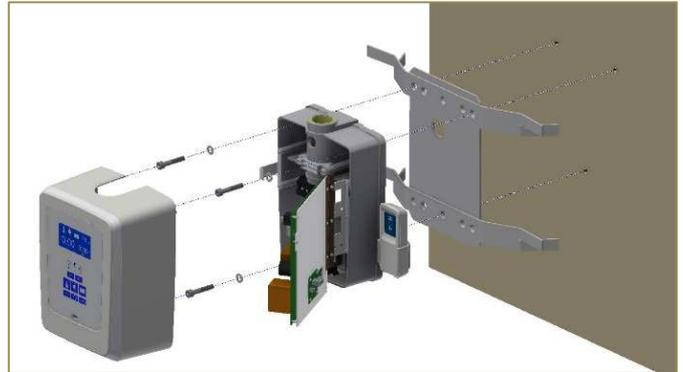
In the case of thin, wood or plasterboard walls, which are not solid enough, it is mandatory to use a steel backing plate, as described in the following image.
