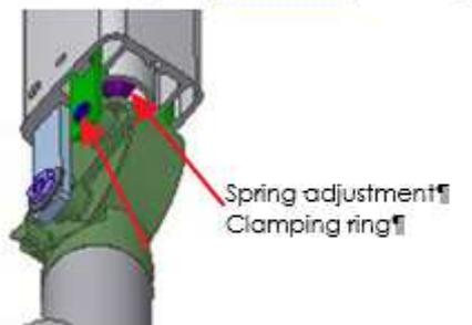
The adjustment must be performed with the first arm in a vertical position and the second arm open. Using pliers remove the retaining ring and remove the pin from its seat to allow access to the spring adjustment.
