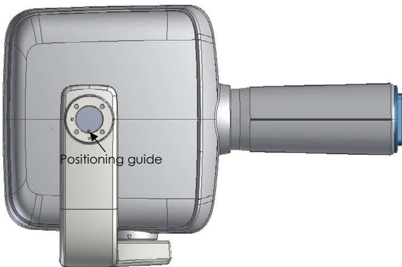
The positioning guide is a reference to facilitate the coupling between the monoblock and the arm.
