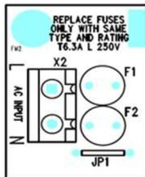
The power board is equipped with two fuses , one of which is bypassed by a resistance wire ( JP1 ) that, in the case of the mobile system , is cut so as to ensure the protection of both the power cables.
