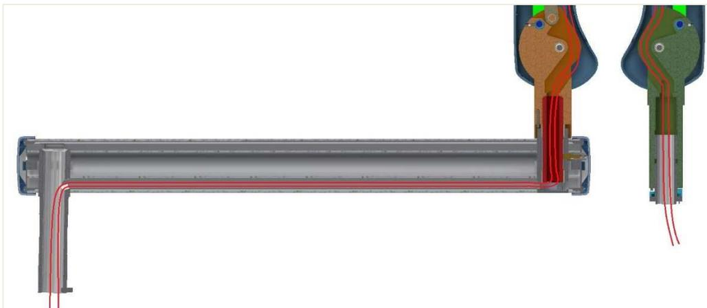
**V1 Model :** place the extension arm directly to the wall plate and after that easily install the scissor arm and connect the cables as shown below.
