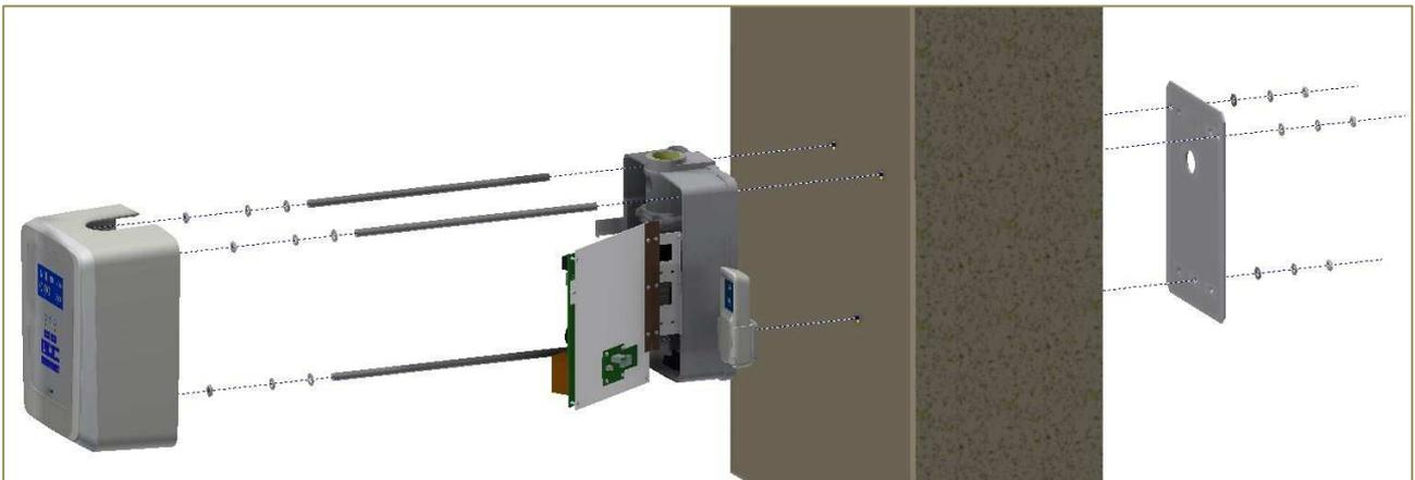
We recommend to install a second backing plate (one plate to each side of the wall) when a single plate is not enough to fasten the equipment.
