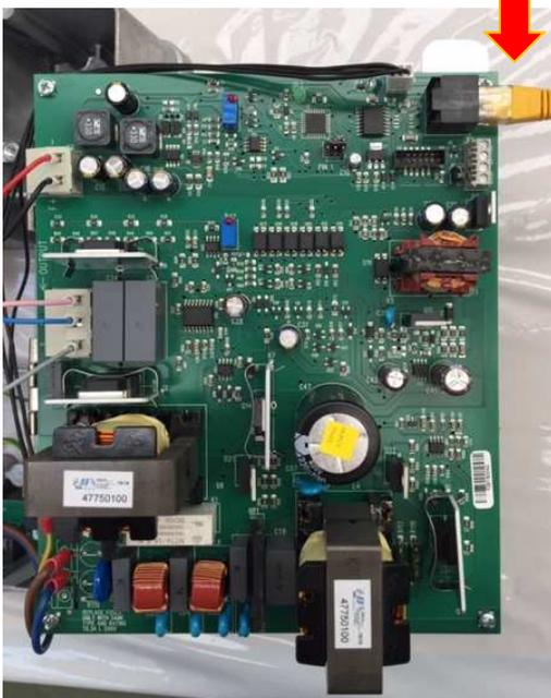
Ethernet cable connection to the remote panel
