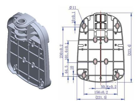
d. Double Stud 16" Wall Plate Adaptor Dimension (measures in mm):
