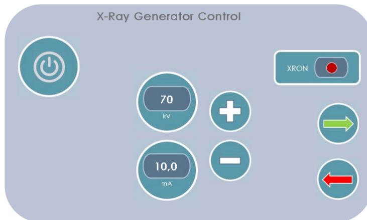
From here it is possible to set the parameters for an examination. Once selected the desired parameters, by pressing the green arrow the screen shows the information for emission process. The screen displays a real-time status of the return signal from the XRPSI card, XRON, and the return values of the feedback of kV and mA, always from the inverter Board.
