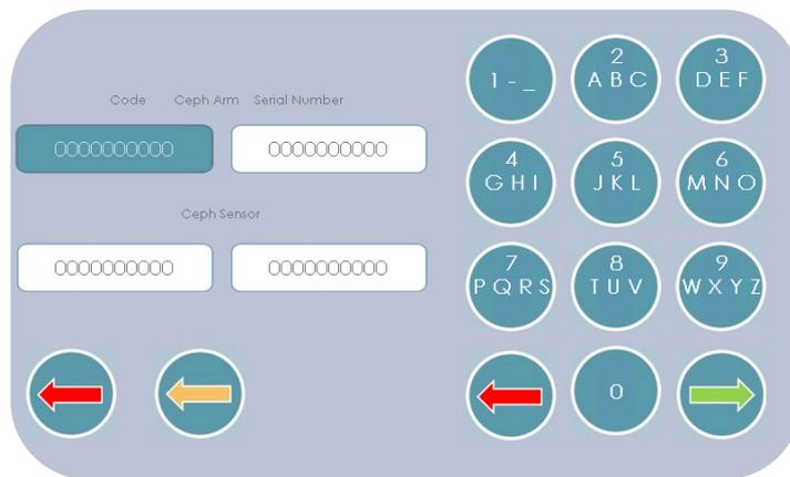
The keyboard has the same logic of a common mobile keypad. By pressing repetitively the same button, it will scroll the number and the letters associated with that key, e.g. pressing button 2 in succession will scroll the number 2 and letters a, b and c. To insert the same character twice, for example twice the number 2, press the button 2, wait 3 sec and press it again.
