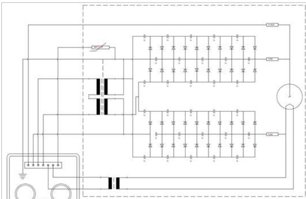
Generator scheme - mA and kV feedback for measurements
