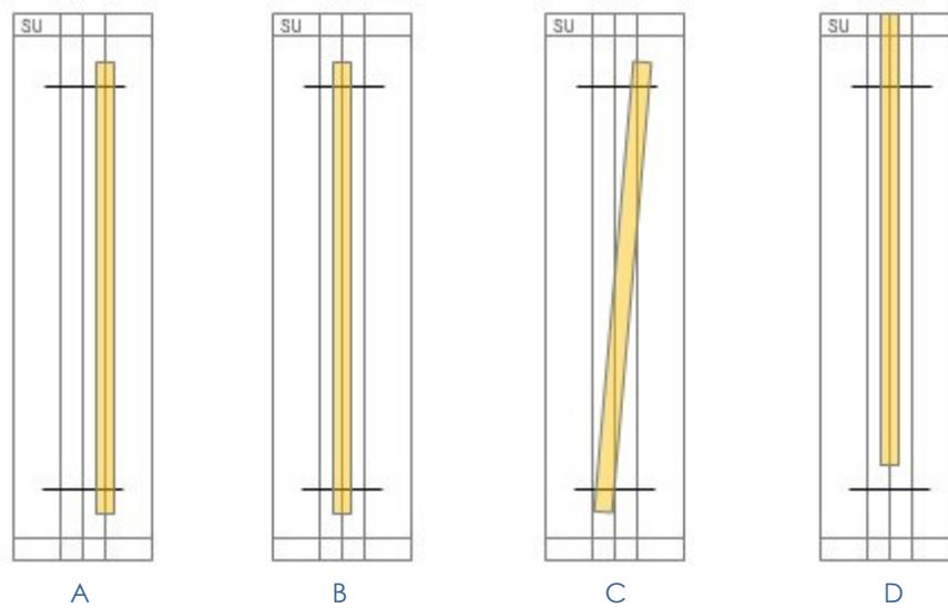
The **optimal centering condition**, which is described in case B, occurs when the exposed field is within the reference area i.e., the highlighted line is perfectly positioned in the middle of the white area.
