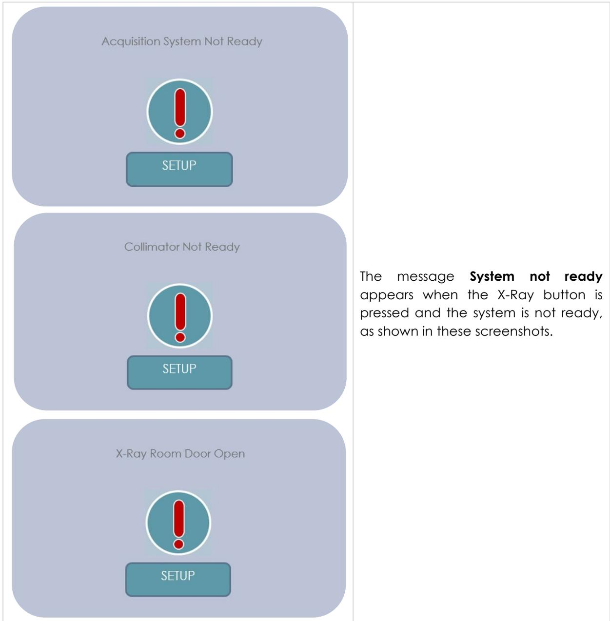
The message **System not ready** appears when the X-Ray button is pressed and the system is not ready, as shown in these screenshots.
