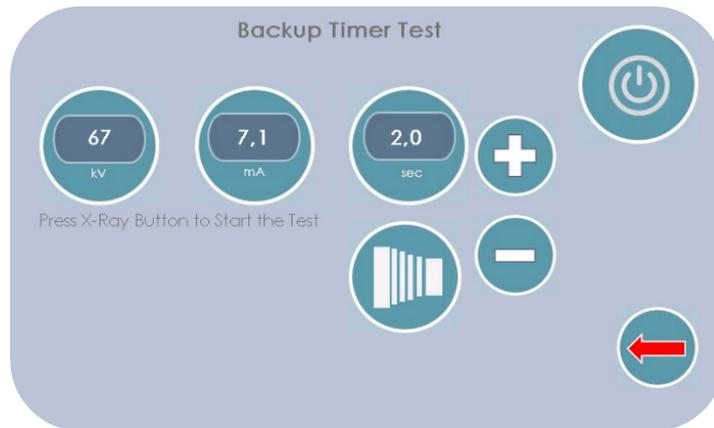
The test is similar to that described for the measurement of the exposure parameters but in this case, the exposure is not interrupted at the end of the set time, but continues until the backup safety timer, verifying the accuracy of the intervention.
