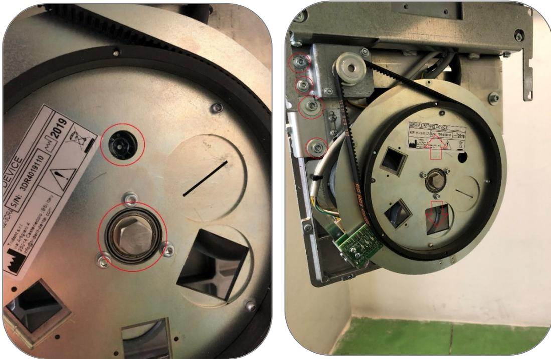
The set screw under the collimator eases the up/down movement. To move the collimator down, slightly loose the screw of the motor to avoid the belt to be tight.
